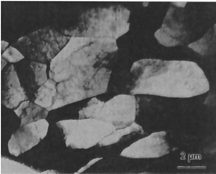
Figure 16.1. TEM-micrograph (X5700) of Silicon-Steel. Reprinted from Axelrad, D. R. (1993) Stochastic Mechanics of Discrete Media , Springer-Verlag Berlin Heidelberg, pp. 64, with kind permission from Springer-Verlag Berlin Heidelberg.
