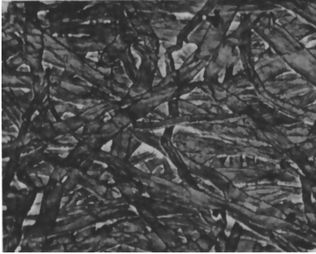
Figure 16.4. SEM-micrograph (X170) of Sulphite-paper (Fibrous structure). Reprinted from Axelrad, D. R. (1993) Stochastic Mechanics of Discrete Media , Springer-Verlag Berlin Heidelberg, pp. 65, with kind permission from Springer-Verlag Berlin Heidelberg.
